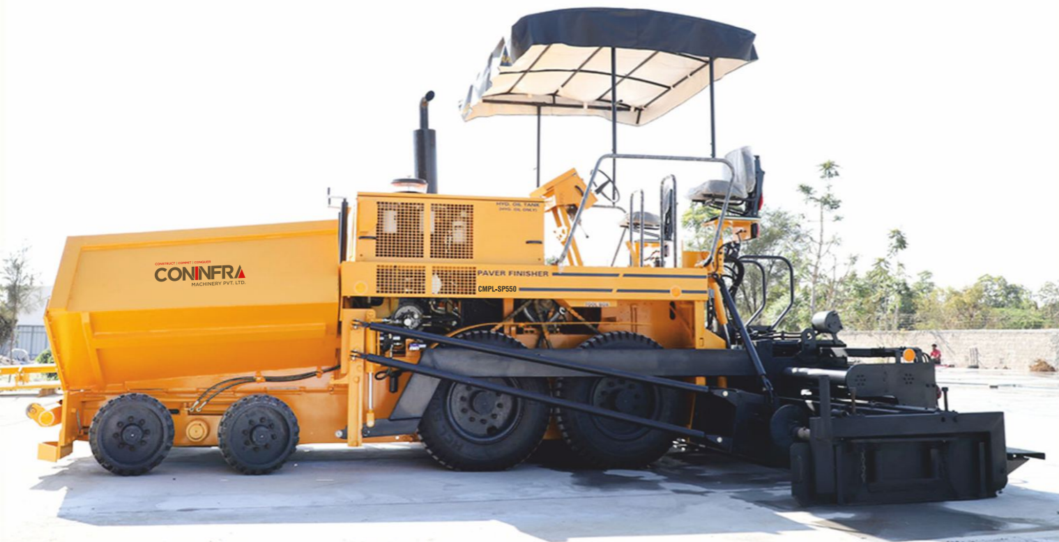
Technical Specifications CMPL-SP550 (Suitable for Bituminous, Wet Mix, GSB, DLC & DBM Material)
