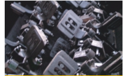
Inside view of Pugmill
